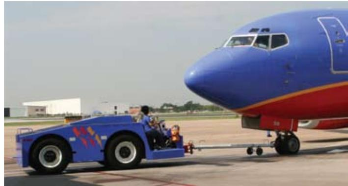
**GSE:** In 1997 Southwest Airlines began to invest in Ground Support Equipment Electrification. There were 701 pieces of equipment electrified by year end 2008, including bag tugs, belt loaders, lavatory trucks, and pushbacks. By using electric power to run the equipment instead of fuel, we estimate we have reduced 2008 ground support equipment fuel consumption by as much as 550,000 gallons and reduced emissions by 5,000 metric tons of carbon dioxide equivalent.
